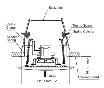
• Make a 157 mm ±2 diameter hole in the ceiling. Making-off pins provided on the mounting bracket will help scribe the circle of its diameter on the ceiling.
